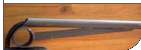
Figure 1 A 12 mm bar bent to correct diameter of 60 mm. Source: CCANZ IB79
